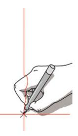
Its long working range with a line length of up to 5 metres means that you don't have to apply it repeatedly like you do with a spirit level. You can immediately mark all of the holes you need to drill along the laser line or you can start to mask straight away.
